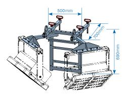
The modular mount for crane lighting is impressive with its simplicity, durability and expandability. It can be fitted on the ground by one person ready for use, and be to the crane. It can be also dismantled into its separate modules, which have been designed to save space.
